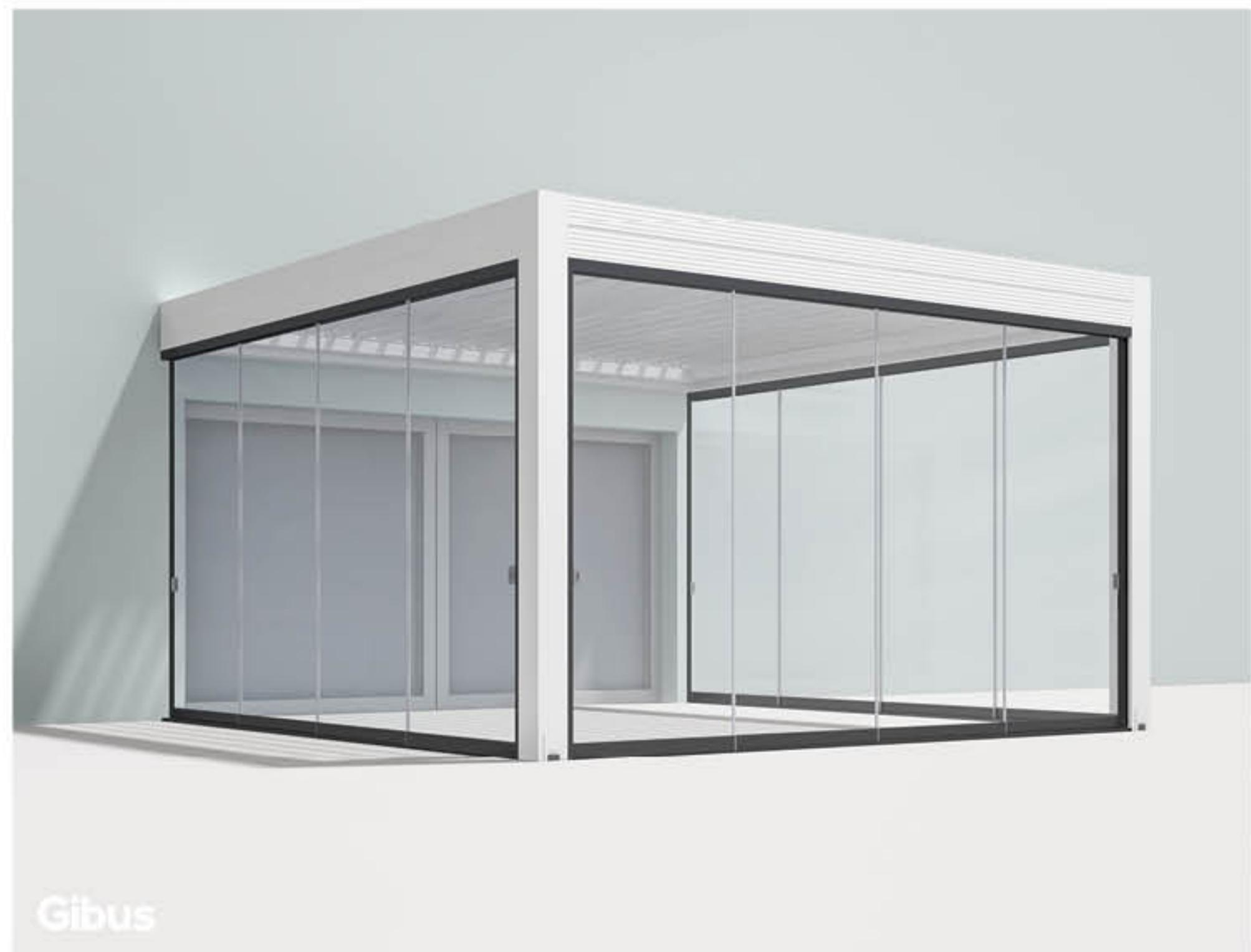
**EN** Glisse is characterized by a high attention to the finish and an accurate choice of materials. It consists of tempered glasses (also available in extra-clear and satin version), powder-coated aluminium structure and rails made of anodized aluminum. Each tempered safety-glass panel (10 or 12 mm) slides on parallel aluminium rails by means of 2 carriages, which allow a smooth and silent movement.
